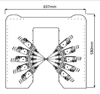
Sample4: Probe Configured with 10 DC Probes
